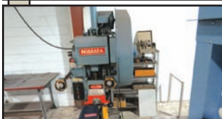
NIAGARA A-22 OBI Non-Geared Gap Frame Press
