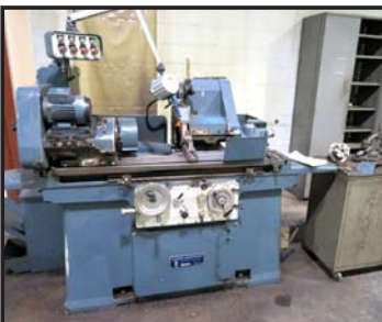
JONES & SHIPMAN mdl. 1300 Universal Cylindrical Grinder
