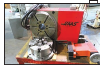
HAAS HRT-310 4th Axis Rotary Table
