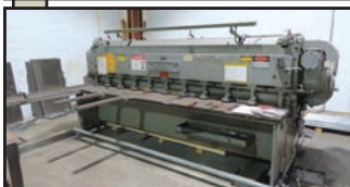
CINCINNATI 1010 Mechanical Squaring Shear
