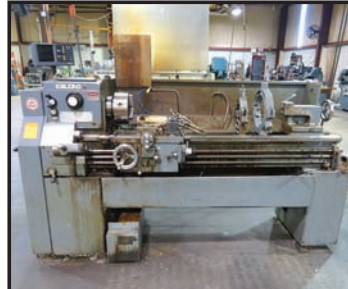
LEBLOND 11C 16x54 Engine Lathe
